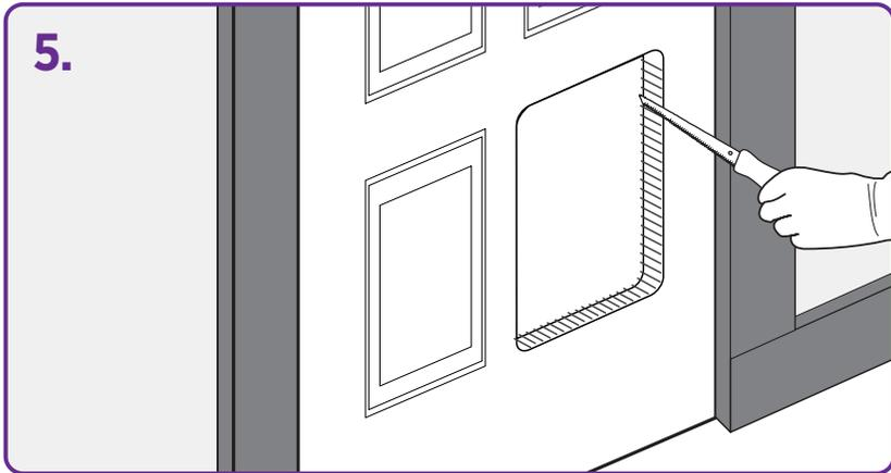
Using a reciprocating jigsaw, cut out the opening, cutting along the pencil outline.
