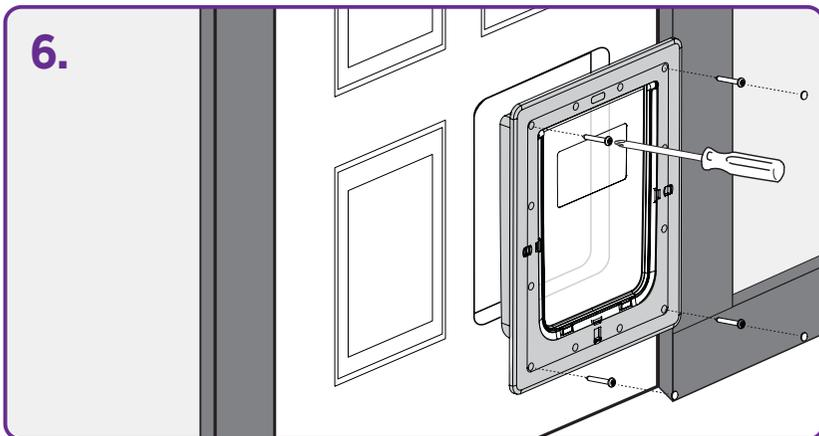
Place both frames into the opening and secure with screws and caps provided.
