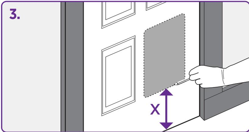
Cut out template supplied in box, line up bottom of cut out with height (x) and trace onto door.
