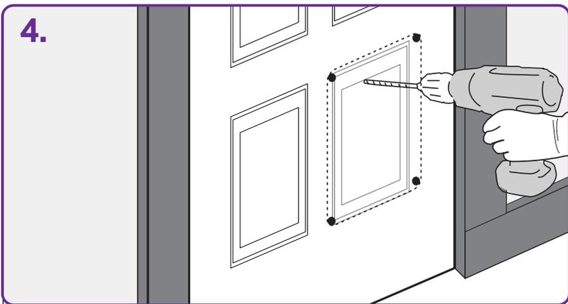
Drill a hole in each of the 4 inside corners with a minimum of 10mm (3/8") drill bit.
