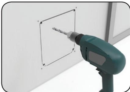
4. Drill holes in each of the inside corners with a minimum of 10mm (3/8") drill bit.
