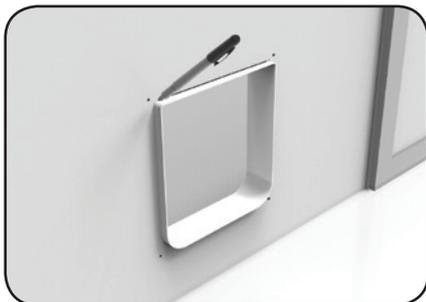
7. Place outer frame in hole, if the tunnel protrudes through the door mark around tunnel.
