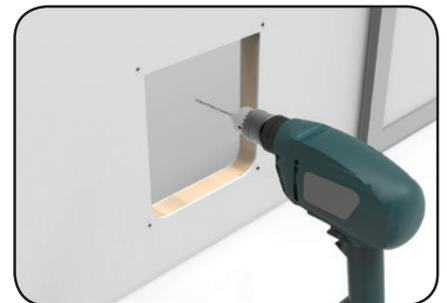
6. Check outer frame fits opening and screw hole align. Drill 3mm pilot holes.
